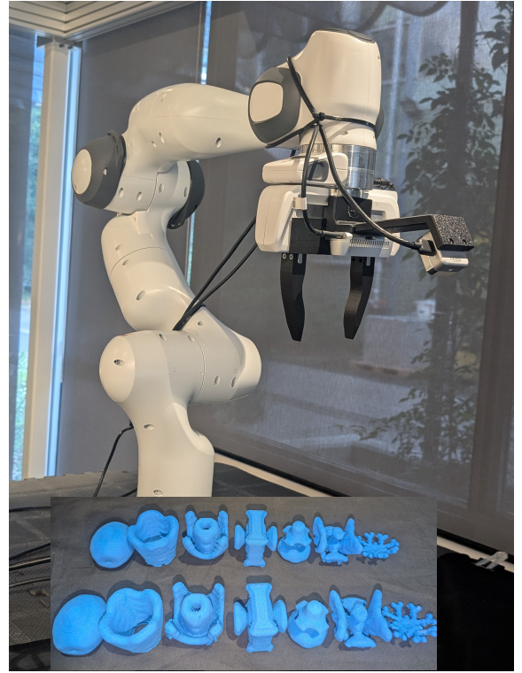
Fig. 1. Experimental setup. The Franka Emika Panda robot is fitted with a parallel-jaw gripper and two wrist-mounted Intel RealSense cameras: a D435 for grasp synthesis from a wider view and a D405 for short-range deformation observation. The inset shows the six 3D-printed EGAD test objects (A0, B1, C2, D3, E4, F5, G6) fabricated in Varioshore TPU; each object is printed at two gyroid infill densities (5% and 20%).
