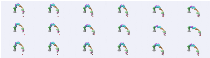
Fig. 4: Simulated Franka push-cube (three trajectories, six time-spaced frames each). The 7-DoF arm is modeled as interacting object-level components and the cube as a free rigid body; both co-evolve under contact. This manipulation regime, with an articulated arm acting on a free object, lies beyond the MOVi free-fall setting and motivates action-conditioned rollout.
